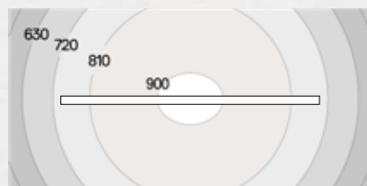
A.39 Sharp microrefractive emission - black louvers 1184 mm - direct only Installation h 2400 mm - Desk h 750 mm Isolines (lx) on a desk 1600x800 mm
